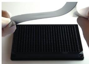
The sealing films may be applied to either the top or bottom of the plate. A split backing aids in applying the sealing film properly. Edge cut-outs assist in positioning and accommodate ribs on the plate bottom.
