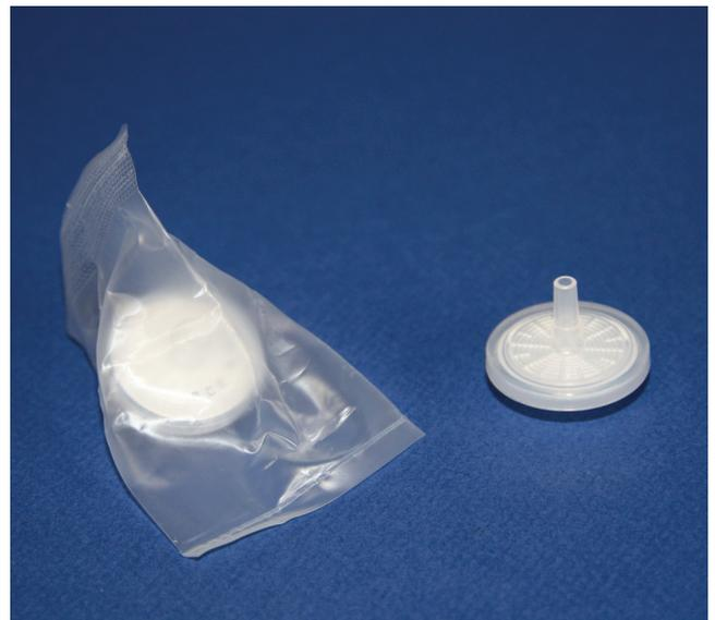
NB. Mycoplasma and some viruses may go through the 0.2µm filter
