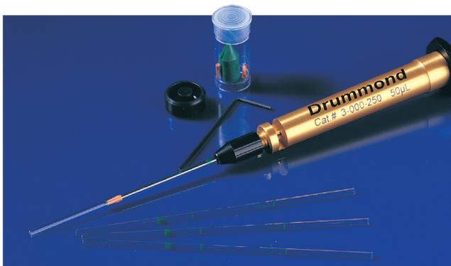
Dialamatic Microdispensers provide precision micro-volume delivery. The stainless steel plungers and borosilicate glass capillaries have a volumetric accuracy of  $\pm 1\%$  at full volume. The adjustable plunger is engraved with a fractional delivery scale in pre-marked increments for direct reading and setting. All microdispensers are supplied with colour-coded capillaries, essential maintenance tools and spare parts.
