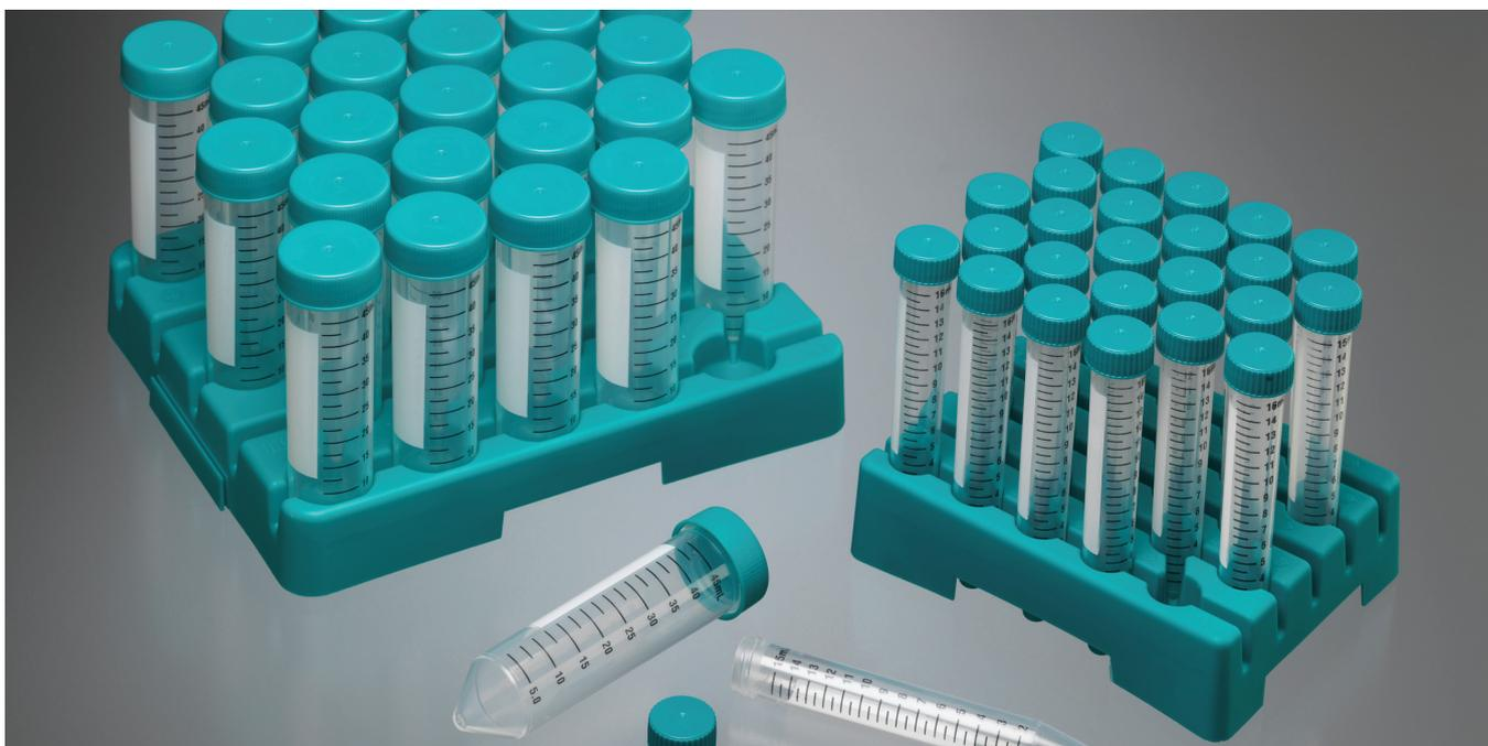
The 50ml tube is available in a free-standing (skirted) format, which allows it to stand upright without the need for a rack. It is ideal for transporting samples since it is lab certified to the IATA 95kPa standard.
