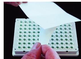
The sealing films may be applied to either the top or bottom of the plate. A split backing aids in applying the sealing film properly. The light-reflective properties of BrightMax plate-sealing films on clear-bottom plates maximize sensitivity of bioluminescence and chemiluminescence assays in bottom-reading luminometers. White films also have an application as a backing matrix for microscopy of punch-out samples from filter plates, for example in ELISPOT assays.
