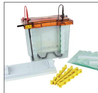
The new Vertical Maxi Z System is the latest product innovation for large format vertical gel electrophoresis. Designed to perform a variety of separations, including first and second-dimension SDS-PAGE, native, preparative, gradient and high-resolution nucleic acid electrophoresis, plus capillary tube gel IEF and electroblotting, the Maxi Z is one of the most versatile maxi vertical systems available.
