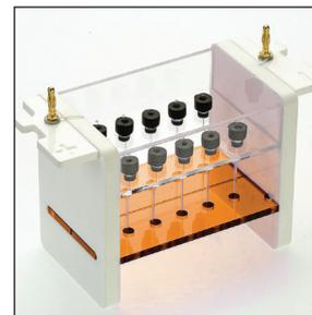
*Clarit-E Tube Gel Units comprise tank and lid, glass capillary tubes, blanking ports and cooling pack.*
