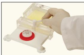
Flexicasters allow the casting of varying gel lengths simply by locking the moveable dam. Adjustable feet and level bubble allow gels of uniform thickness to be poured.
